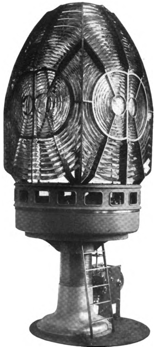
Fig. 55.—Pachena Point Lighthouse, B.C.—First Order Double-Flashing Apparatus.
